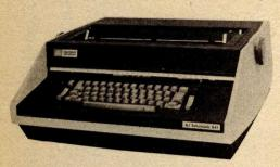
Anderson Jacobson has announced an RS-232 serial interface for their AJ841 IO terminal. This option includes such features as selectable data transmission rates of 110 to 1200 bps; an 896 character receive and print buffer and X-on/X-off control characters to and from the computer.
