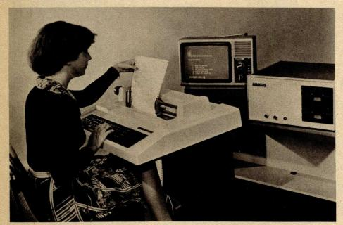
The Abacus 1 is a complete hardware and software package designed to handle basic accounting for small businesses. It includes a Z-80 processor, dual North Star floppy disk system, video display, keyboard and printer, plus software.
