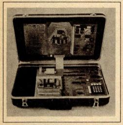
The TDS-M68 microcomputer training and development system offers the personal computer enthusiast an integrated system complete with microcomputer, self-teaching lab manual, text-book and experimenter's lab package. This complete and self-contained system brings together all the ingredients needed for a hands-on training course aimed at
